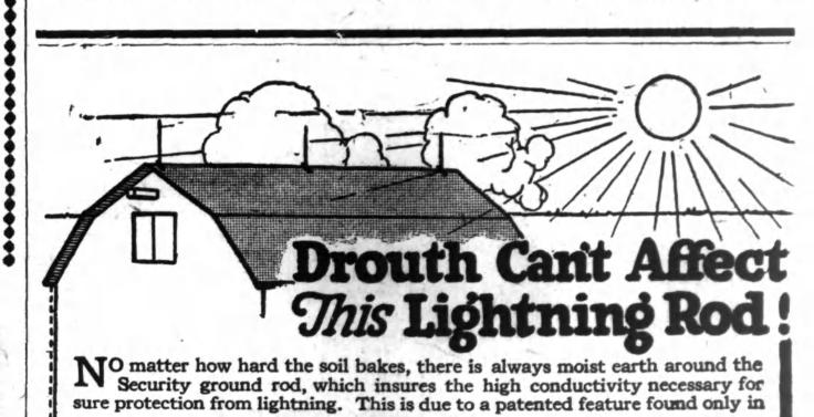
The rod is grounded in a water-filled copper tube. Overflow from this tube moistens the soil and keeps it moist. You never have to pour water on ground rod and you always know the Security will give you protection. Security cable is 99.8% pure and guaranteed free from corroding acids.
