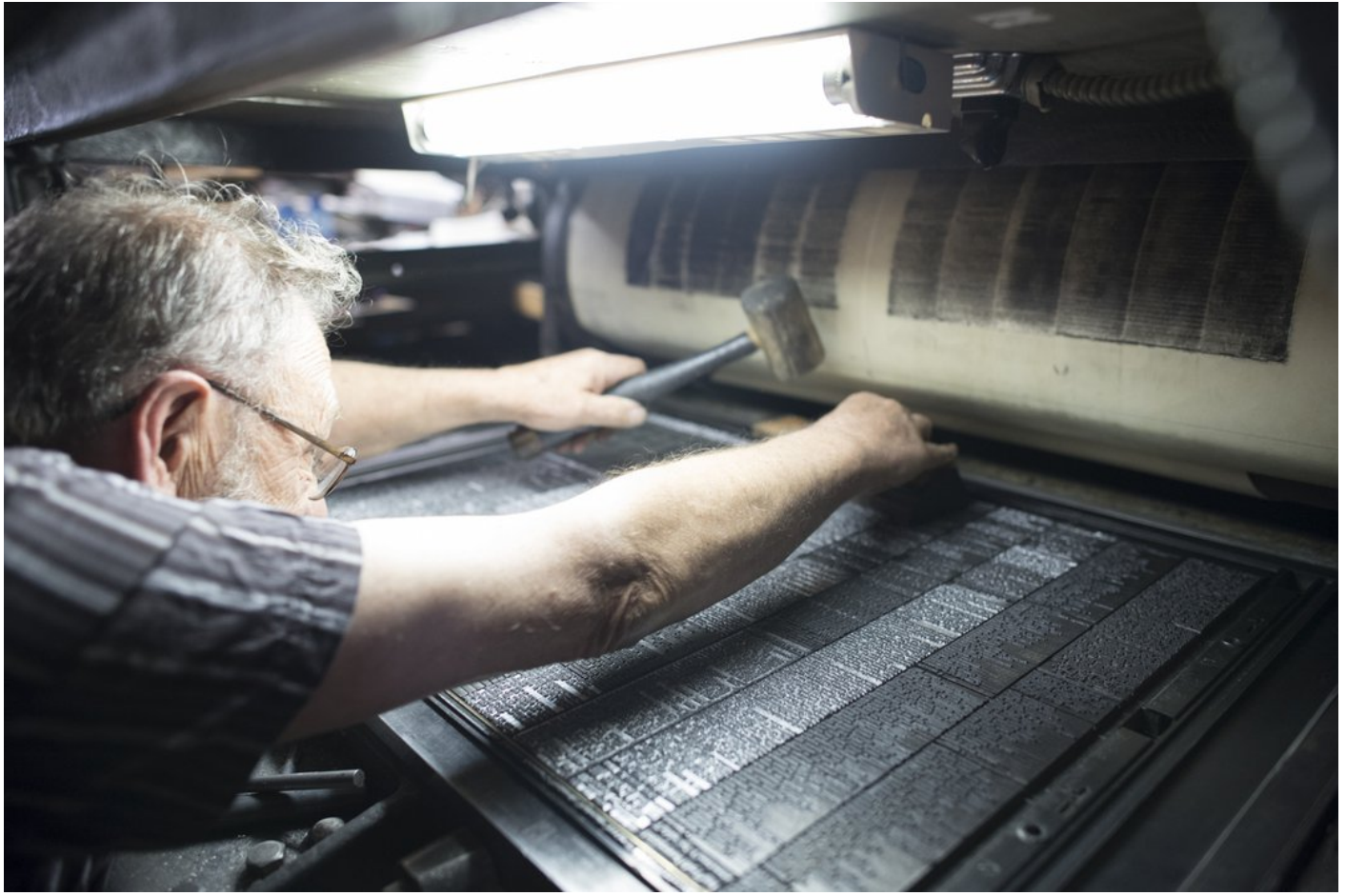
Coombs taps a lead slug in place. Rob Hammer
